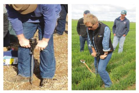
Using a penetrometer in the field to test compaction.
