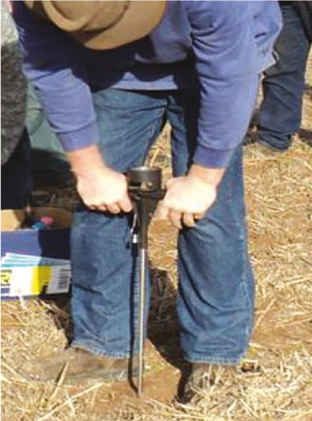
Using a penetrometer in the field to test compaction.
