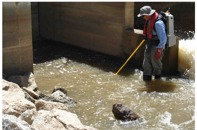
Fish ecologist Clayton Sharpe surveying fish accumulated at Koondrook Weir (downstream) using a backpack electrofisher. Photo: Clayton Sharpe.
