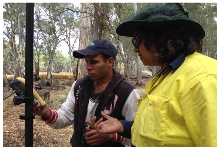
Sharnie and Tom record a site using Differential GPS.
