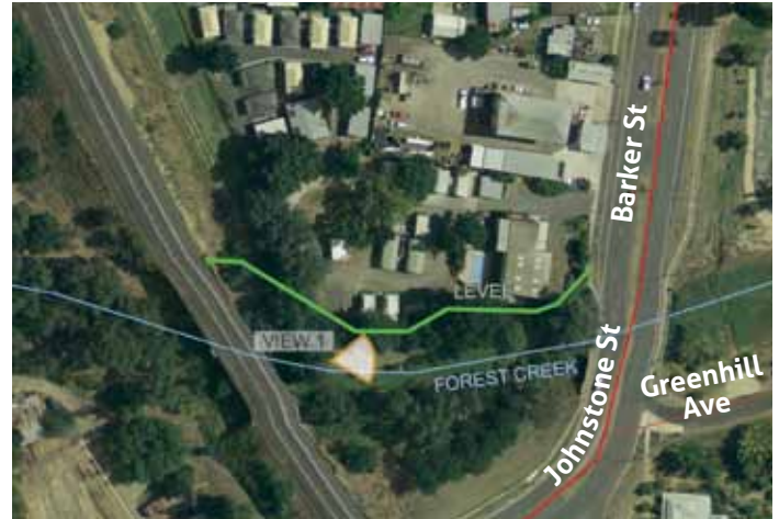
Levee location plan
