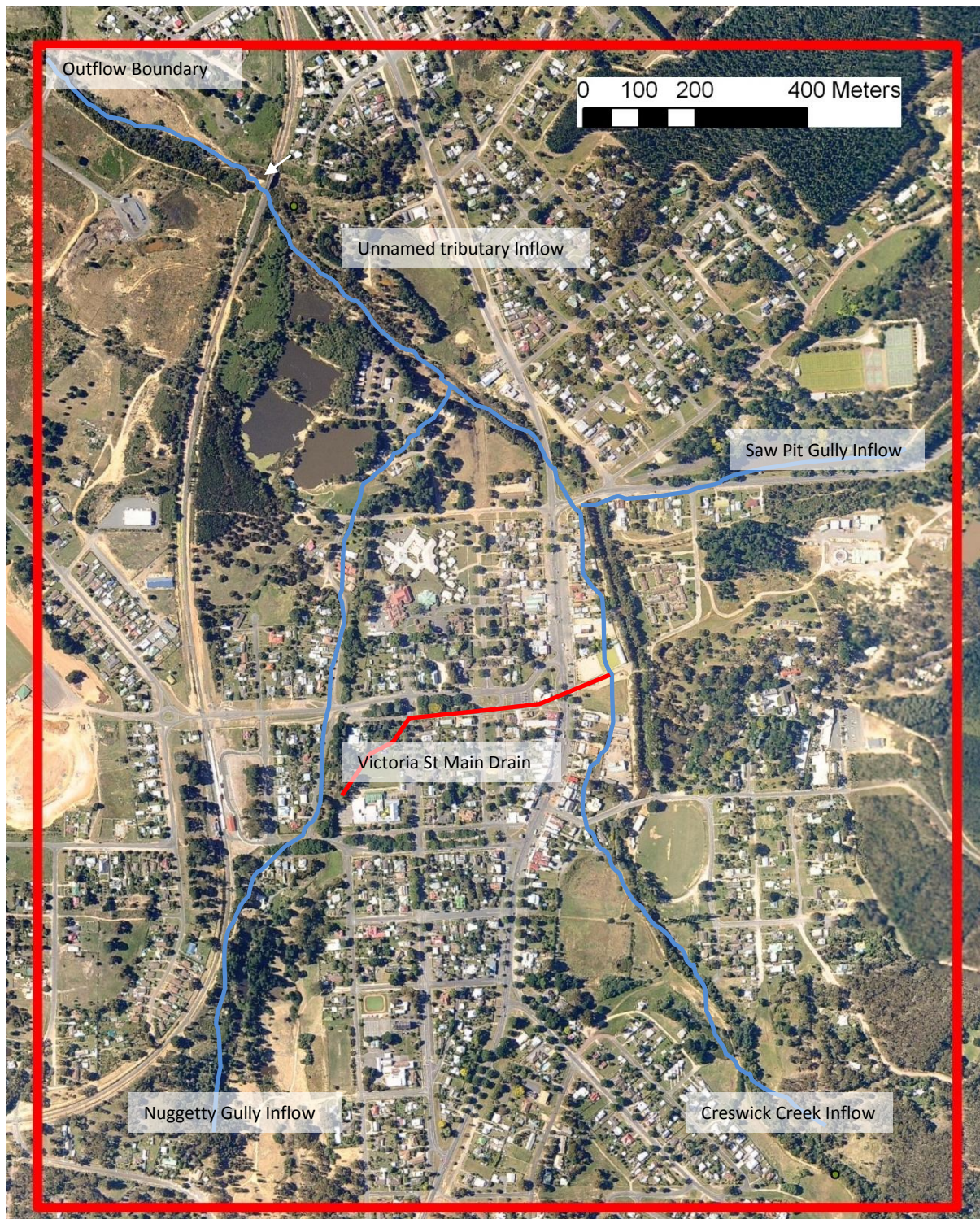
Figure 5-2 Conceptual hydraulic model extents and boundary locations
