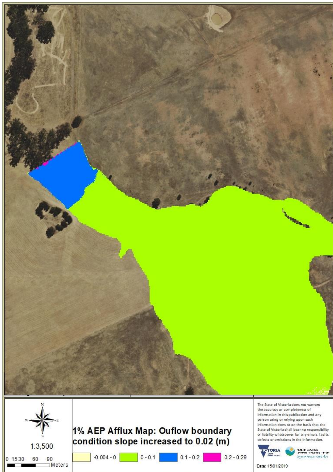
Figure 4.12 1% AEP afflux map comparing base case scenario with sensitivity scenario with the outflow boundary slope increased to 0.02 (Sensitivity Scenario – Base Case Scenario)
