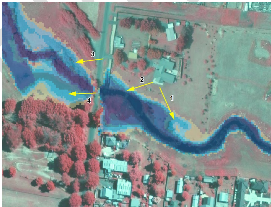
Figure 4-17 Modelled flood extent of the September 2010 event at Wedge Street. Approximate direction of the following photos is indicated by yellow arrows.
