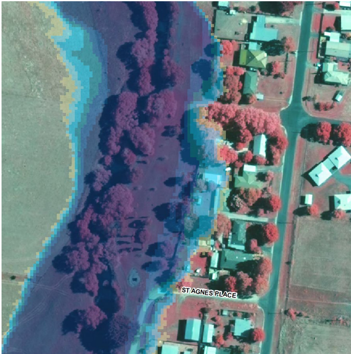
Figure 4-11 Modelled flood extent of the January 2011 event along rear of properties north of St Agnes Place
