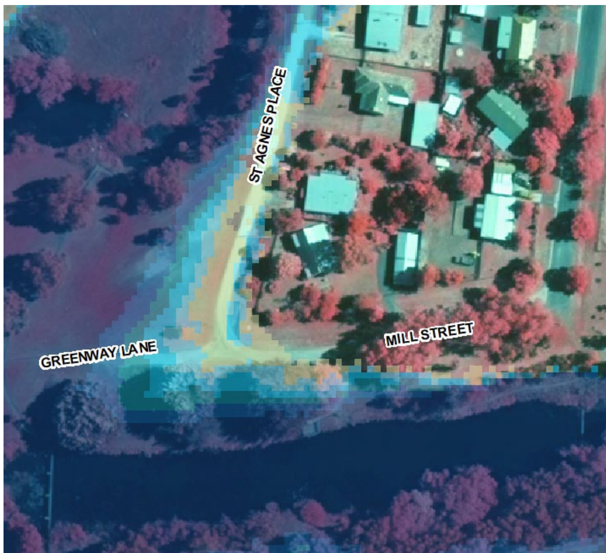
Figure 4-10 Modelled flood extent of the January 2011 event along Mill Street
