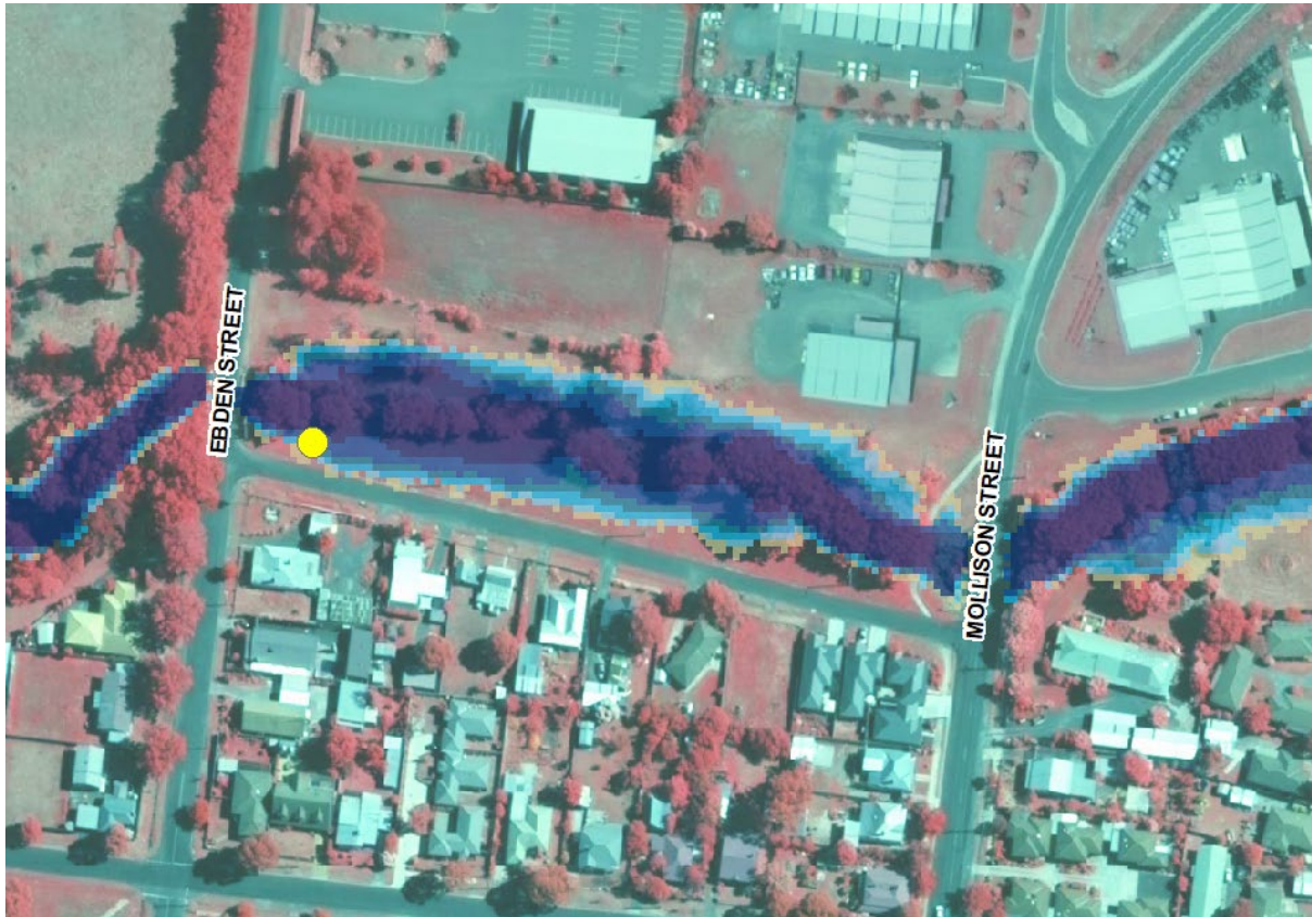
Figure 4-15 Modelled flood extent of the January 2011 event on Post Office Creek. Location of surveyed flood mark is shown as a yellow dot
