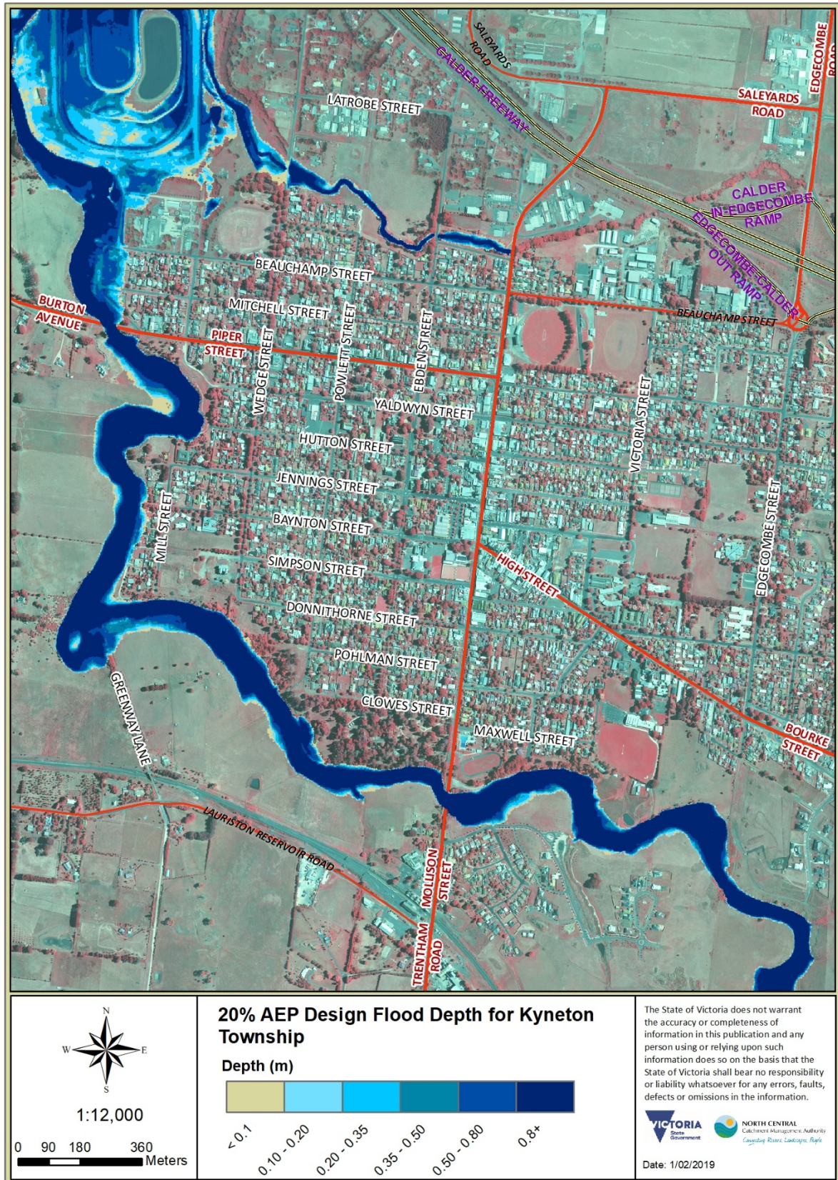
Figure 7-2 20% AEP design flood depth for Kyneton Township
