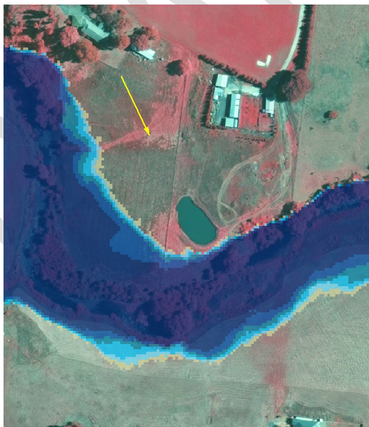
Figure 4-7 Modelled flood extent of the January 2011 event at the rear of Sacred Heart College. Approximate direction of photo in Figure 4.4 indicated by yellow arrow
