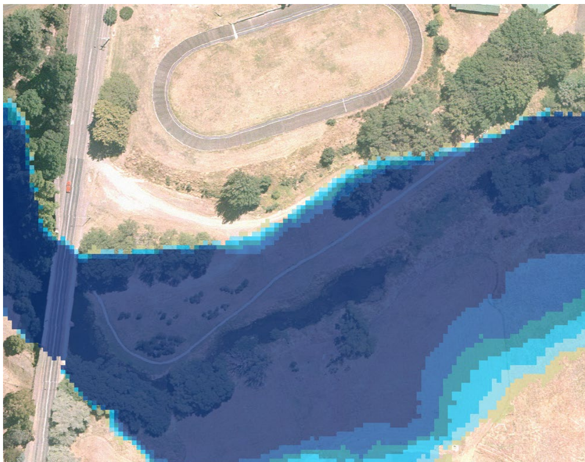
Figure 4-8 Modelled flood extent of the January 2011 event upstream of Mollison Street Bridge
