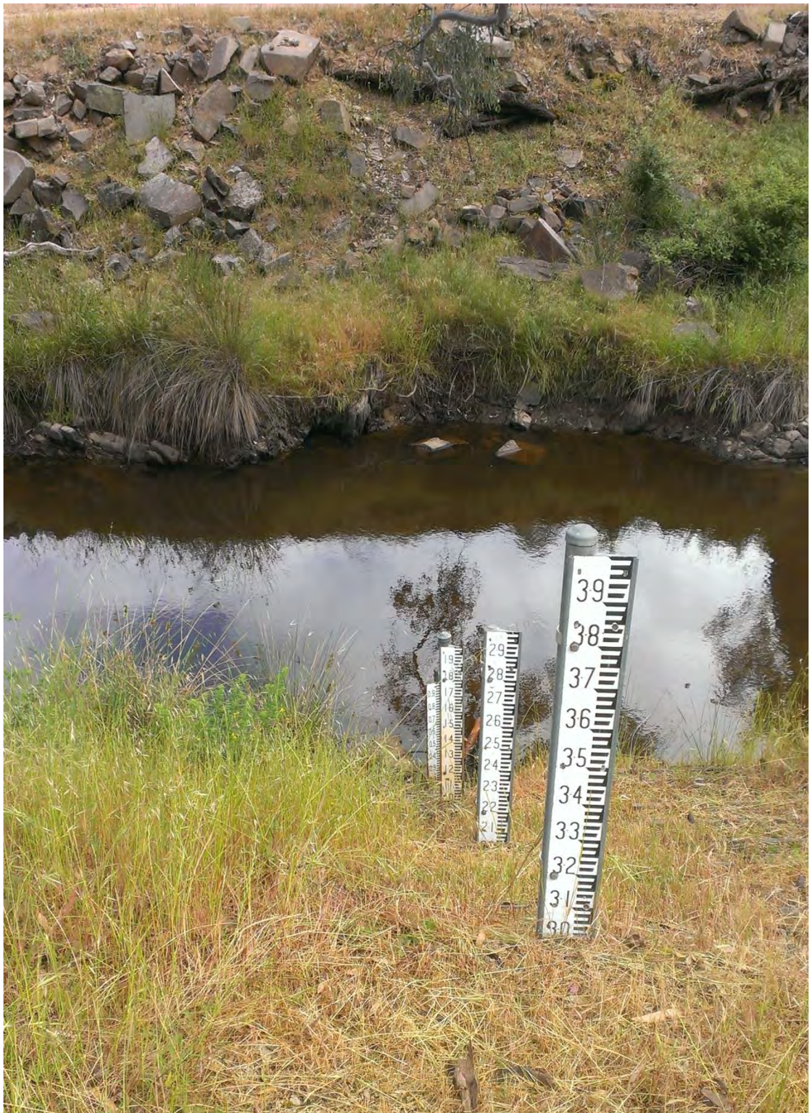
Figure 4-7 Mount Ida Creek Gauge – Gauge Staffs
