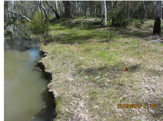
*Erosion pins at the Narrows, Gunbower Creek.*
