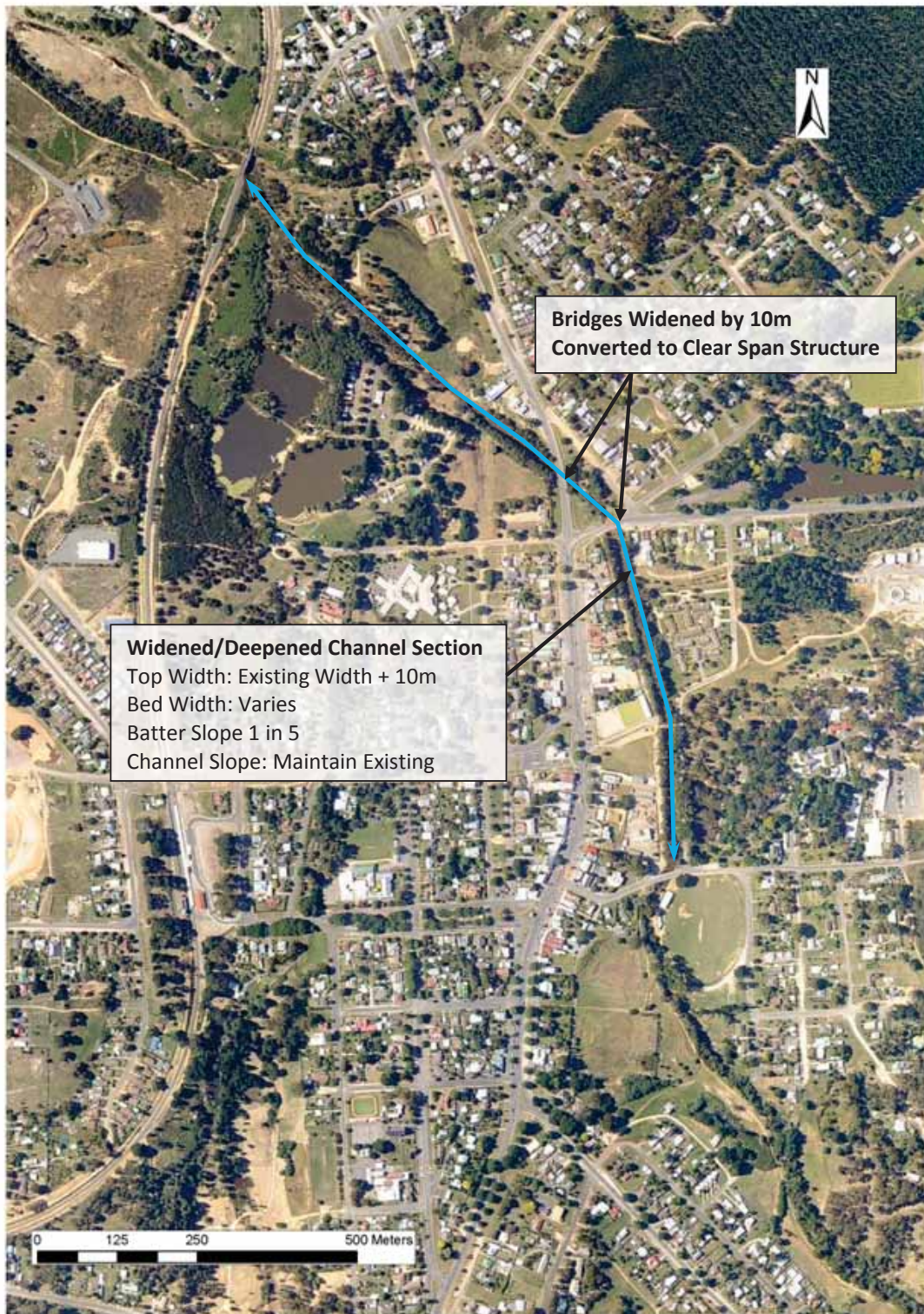
Figure 6-3 Proposed structural mitigation option 2
