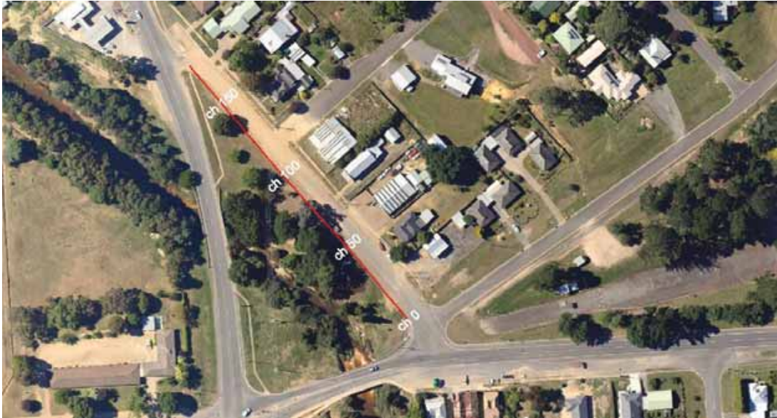
Figure D-8 North Parade Levee Alignment
