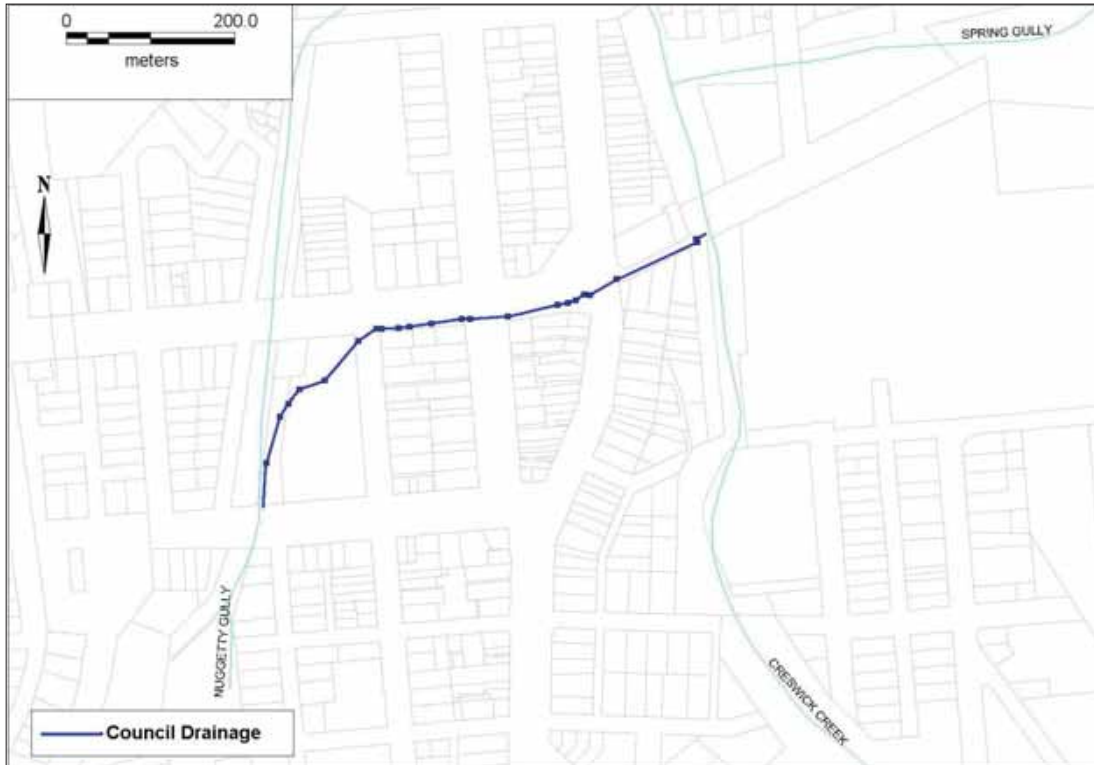
Figure A 1 Location of key pipe network in Creswick included in the hydraulic model
