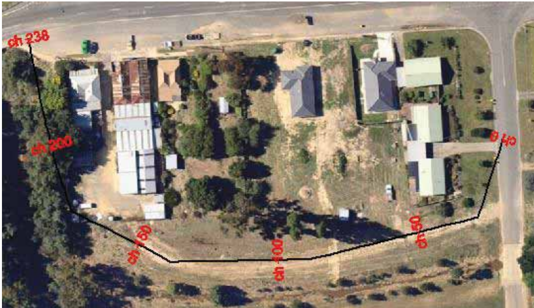
Figure D-4 Saw Pit Gully Levee Alignment
