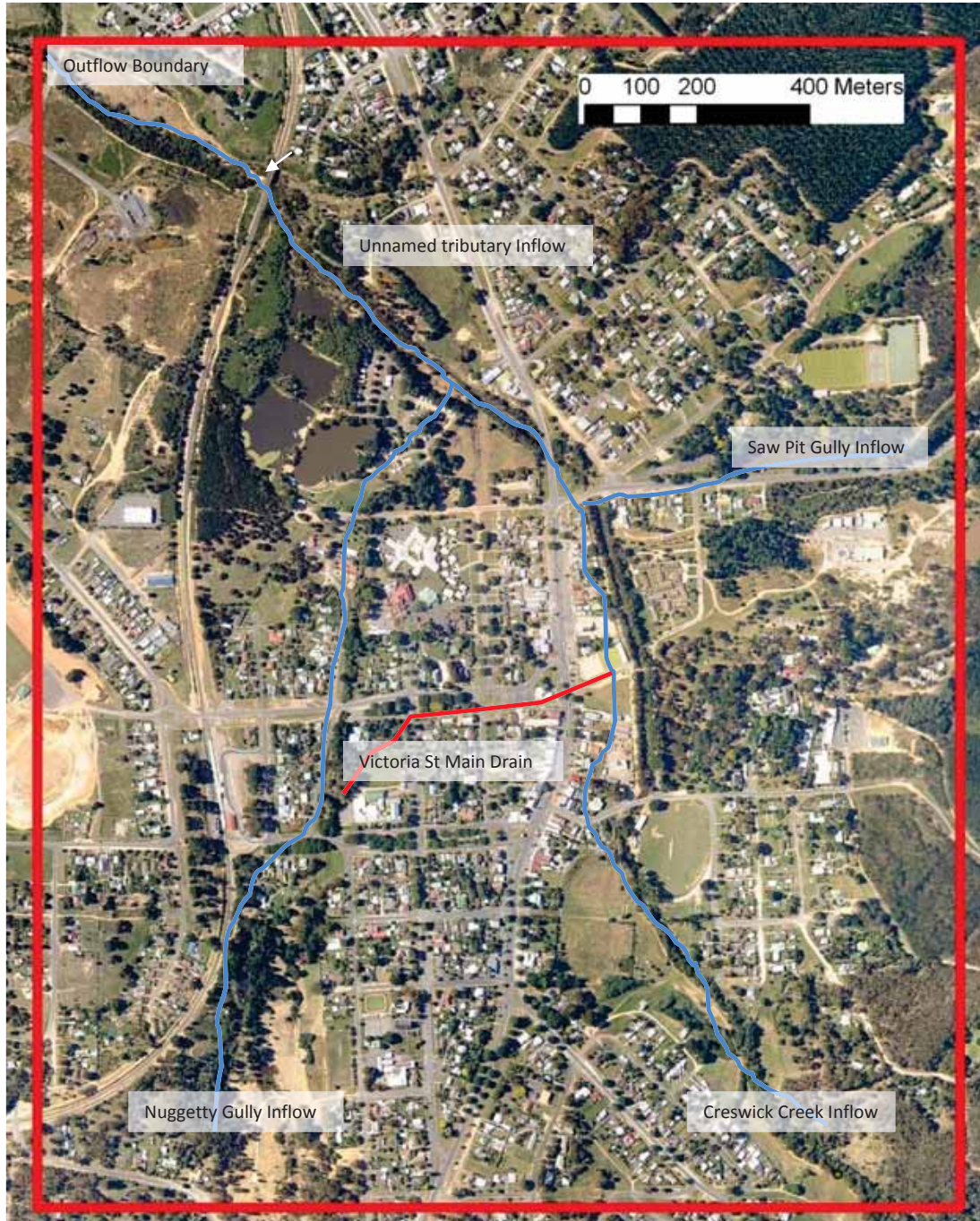
Figure 5-2 Conceptual hydraulic model extents and boundary locations
