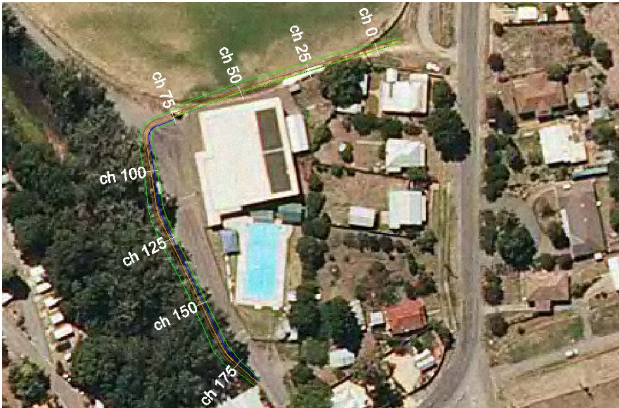
Figure C - 1 Mitigation Option 1 – Right Bank Levee Alignment
