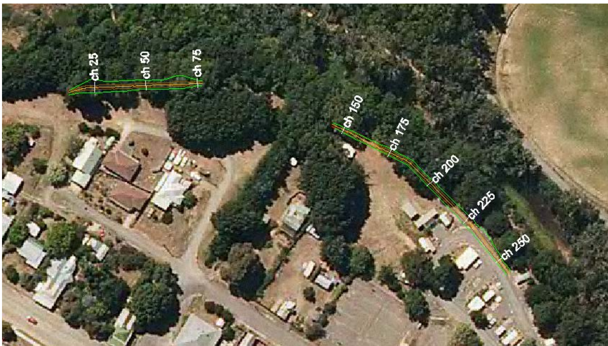
Figure C - 2 Mitigation Option 1 – Left Bank Levee Alignment
