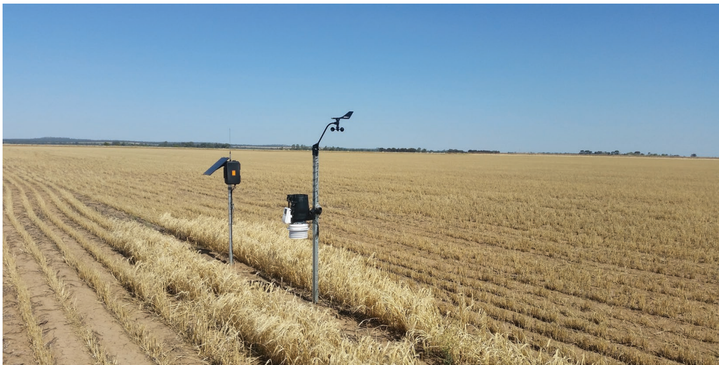
Weather station and moisture probe
