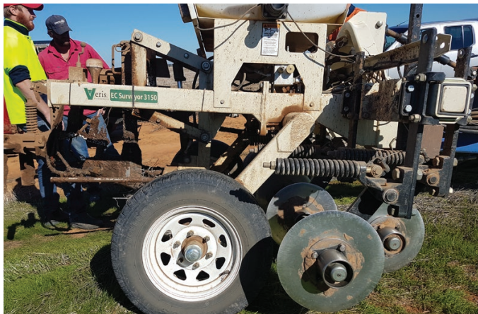
Soil monitoring machine - tests for salinity and pH, and maps the soil
