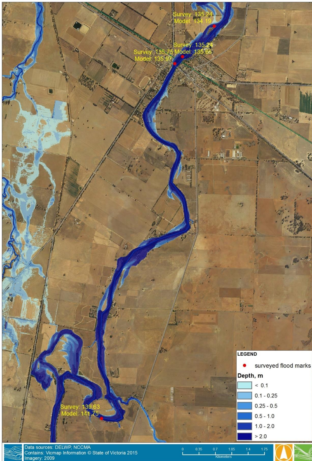
Figure 4-13 Surveyed and modelled flood levels for September 1983 flood event
