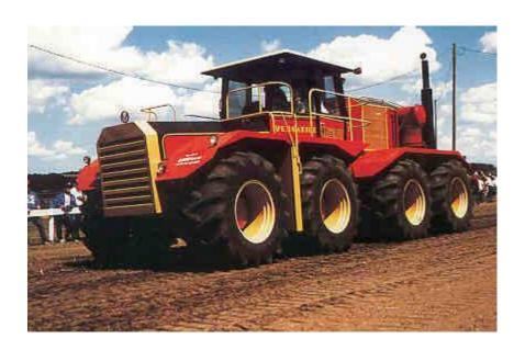
The Versatile 1080 (affectionately know at Versatile as BIG ROY) was built in the late 70s as a prototype. It was a 26-ton, 600hp, eight-wheel-drive monster with a 19-litre Cummins engine in the rear and the 2,100-litre fuel tank in the front section.
