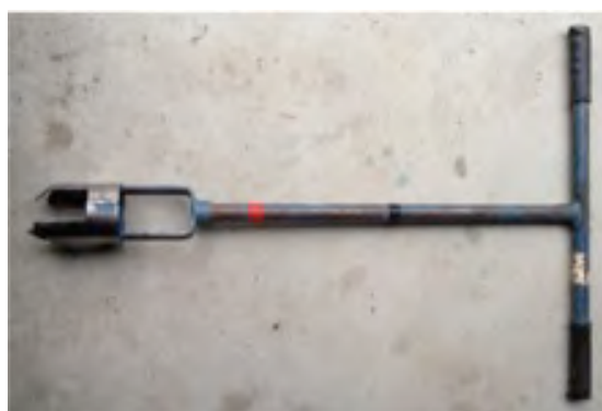
Figure 6-2: Subsoil sampler (four-inch hand auger)
