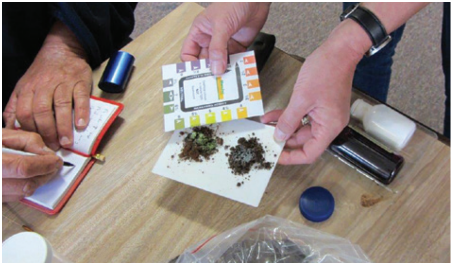
Color chart is used to read soil pH values.
