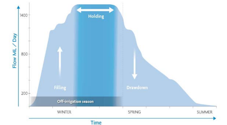
Hydrograph of how the Hipwell Road Channel will be operated this year.
